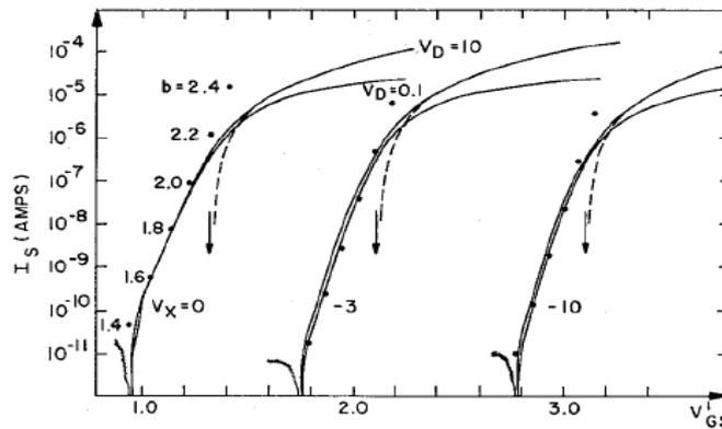
**Fig. 5 Experimental subthreshold characteristics for a long-channel device ( $L = 15.5 \mu\text{m}$ ), [2].**
