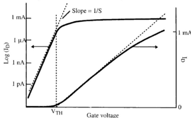
**Fig. 9 Drain current in both linear and logarithmic scales ( $V_{DS}$  is small)**
