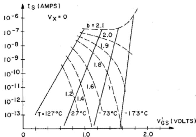
**Fig. 8 Dependence of subthreshold current on temperature for  $t_{ox} = 570 \text{ \AA}$ ,  $N_B = 5.6 \times 10^{15} \text{ cm}^{-3}$  and  $V_x = 0$ , [2]**
