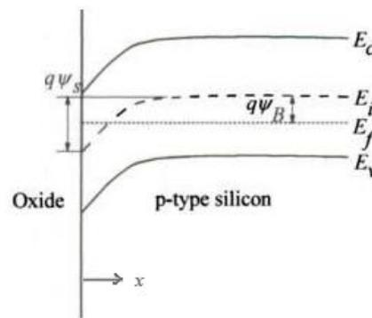
Fig. 2 Energy-band diagram near the silicon surface of a p-type MOS device.
