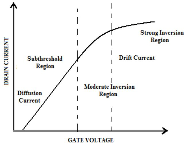
Fig. 1 The three regions of transistor operation shown on a plot of drain current versus gate voltage. The threshold voltage occurs in the transition region.
