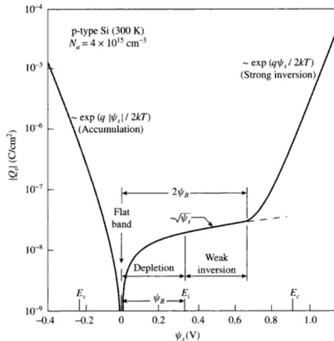
**Fig. 3 Variation of total charge density (fixed plus mobile) in silicon as a function of surface potential for a p-type MOS device, [7].**
