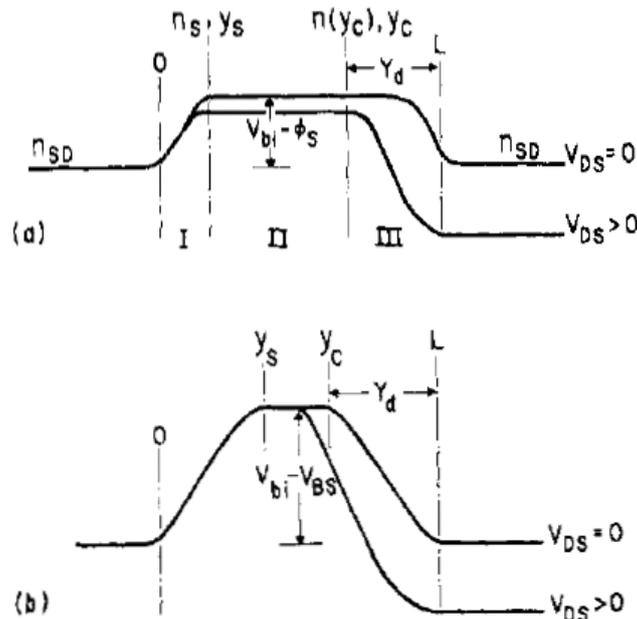
**Fig. 7 MOS device and associated channel potential in the subthreshold region (a) at the surface and (b) below the surface. [9]**
