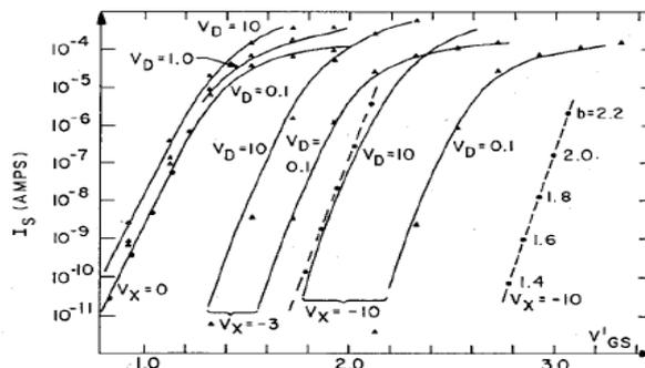
**Fig. 6 Experimental subthreshold characteristics for a short-channel device ( $L = 2.1 \mu m$ ). Points shown are calculated from One-dimensional model and the triangles from two-dimensional model [2].**
