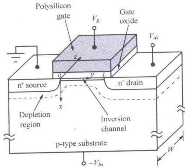
**Fig. 4 A schematic MOSFET cross section showing the axes of co-ordinates and the bias voltages.**
