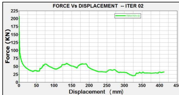
Figure 26: Force Vs Displacement (Energy Absorbed by Material) for Iteration 2
