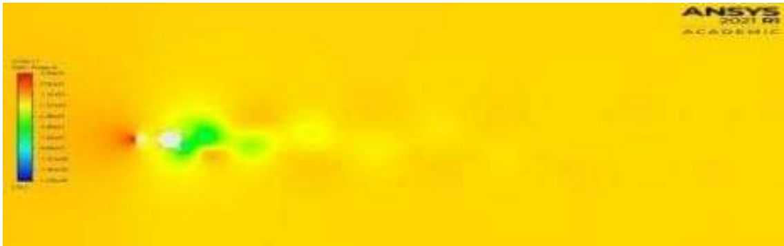
(b) Pressure contour at Re 180 where d=0.5D
