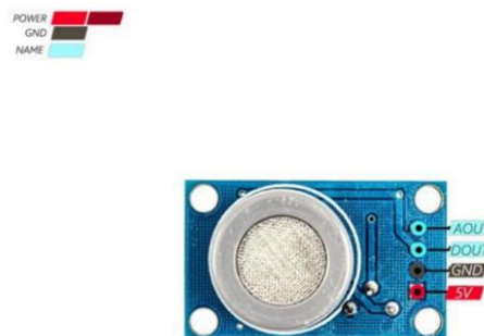
Figure 4: Pin diagram of MQ7
