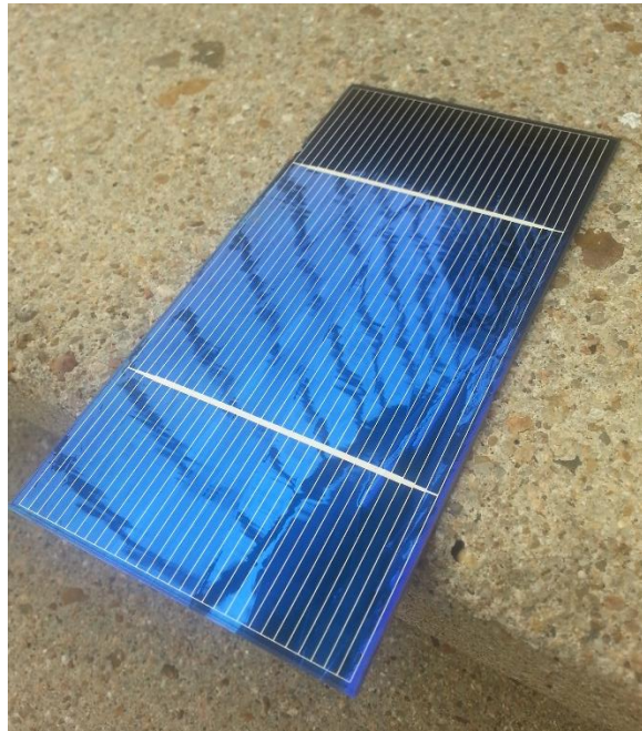
Figure - Actual Solar Cell used in this project
