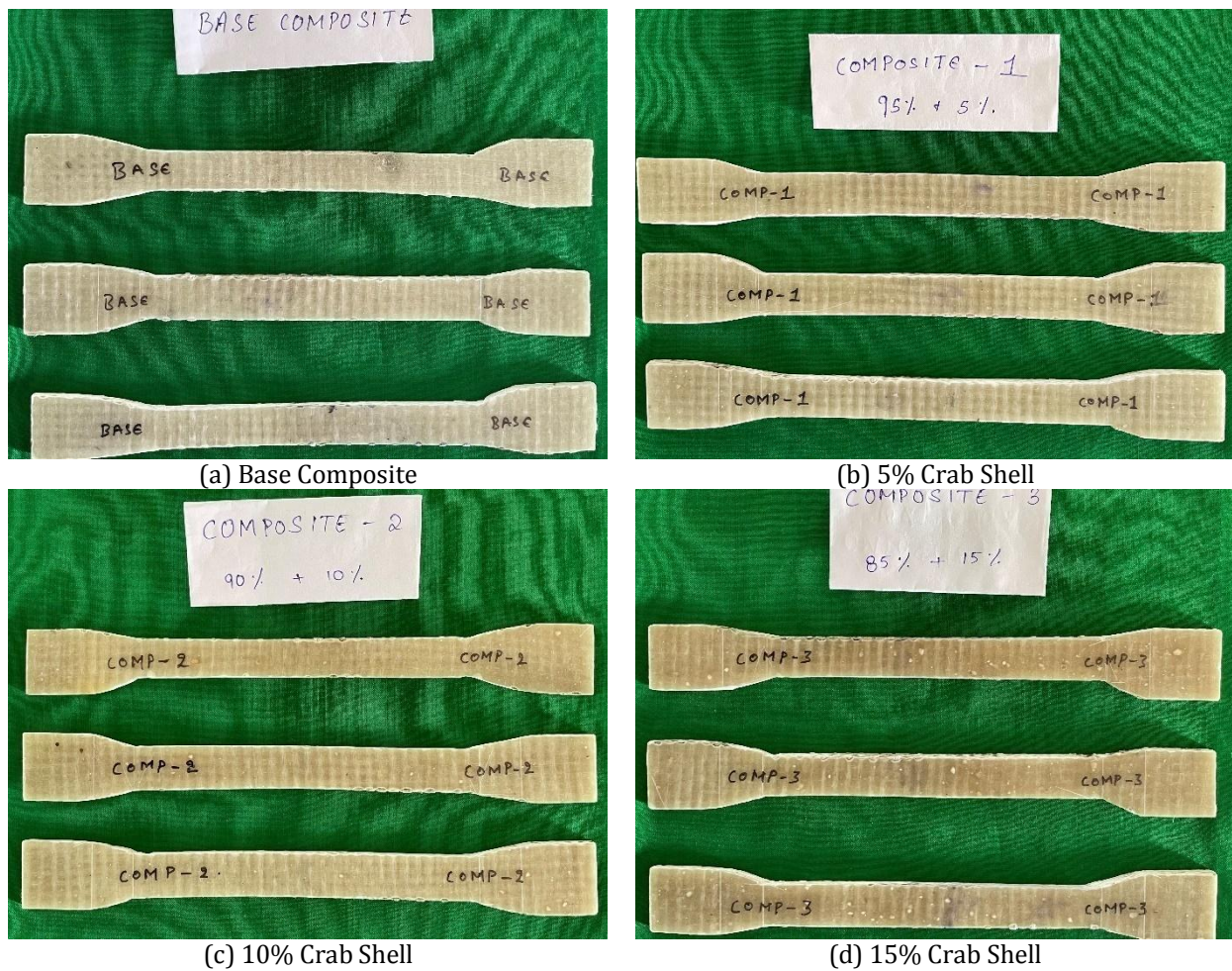
FIG 3.1: (a, b, c, d) tensile test samples of the respective composite materials.
