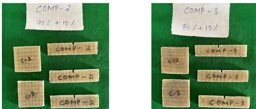
(c) 10% Crab Shell (d) 15% Crab Shell FIG 3.2: (a, b, c, d) Hardness & Impact samples of the respective composite materials.
