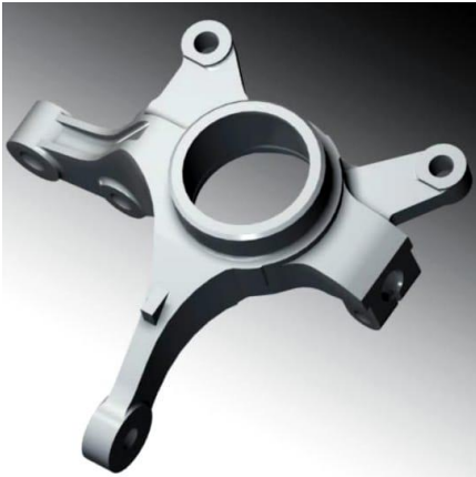
Fig1. Isometric view of a steering knuckle
