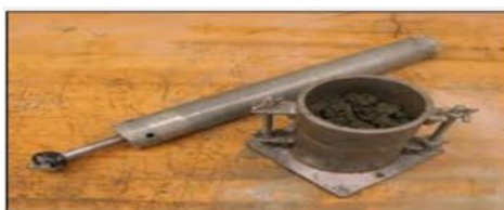
FIG 6 STANDARD PROCTOR TEST APPARATUS
