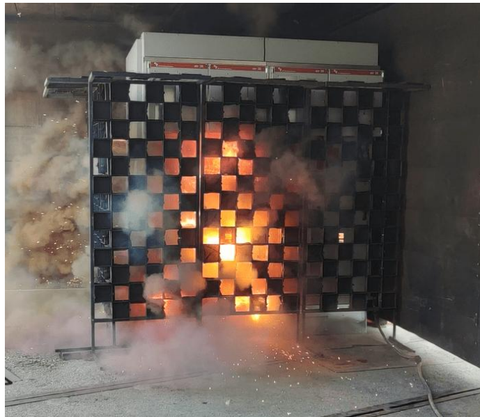
Figure 2 - Event of an internal arc fault
