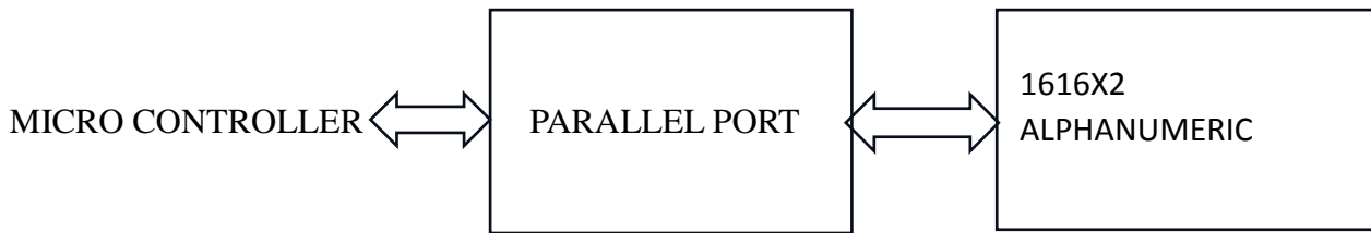
Fig 3.3: 16x2 LCD connection to microcontroller
