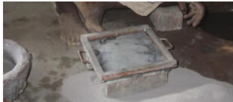
Fig.2.1.3 Metal frame that serves as a boundary box is attached to a base of glass
