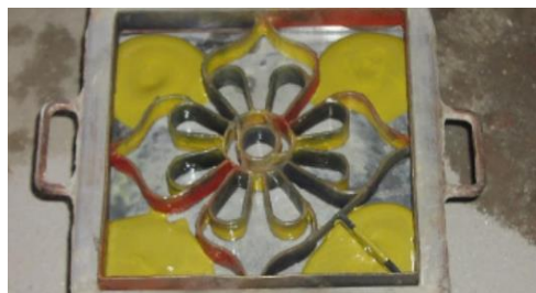
Fig.2.1.5 Various coloured mixtures are poured into the various stencilled areas with ladles
