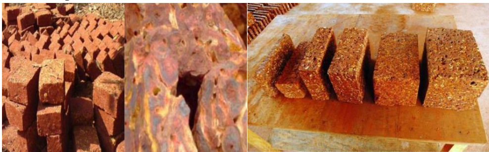
Fig.2.5.1 Colours, patterns in laterite and their use as masonry blocks – cut in different sizes
