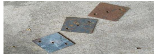
Drilled Mild Steel plates
