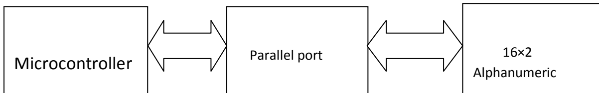
Fig 4.3: 16×2 LCD connection to microcontroller
