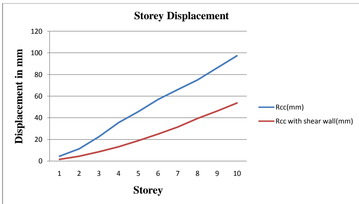
Fig 19: Graph plotted of Lateral displacement comparing both RCC building model
