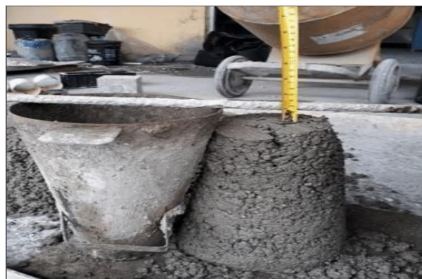
Fig. 4 – Slump Cone Test Performance
