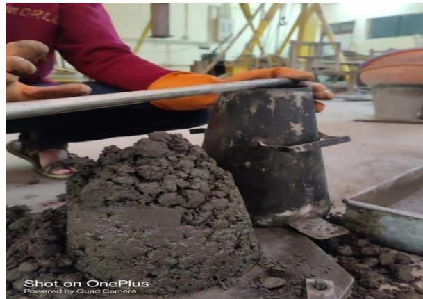
Fig VI: Slump test to determine the workability of concrete
