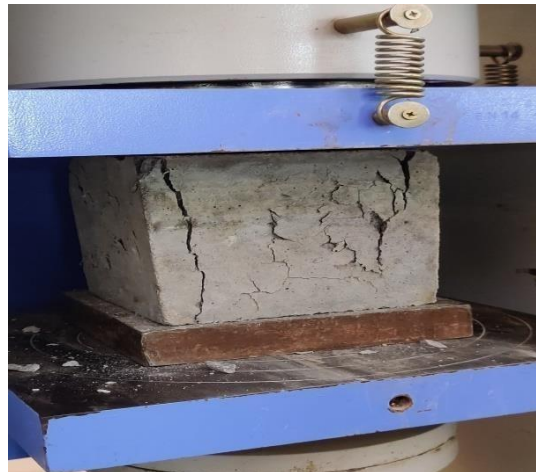
Fig IX: Failed specimen under compression test
