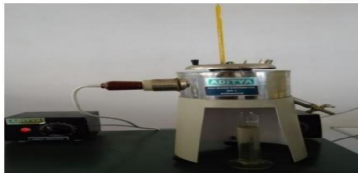
Figure .5 Redwood viscometer
