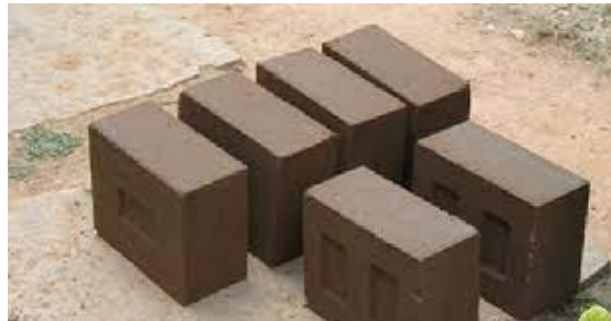
Fig1: Stabilized mud block masonry
