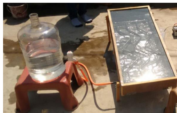
Figure 3 Assembly of Solar Water Heater
