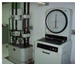
Figure 11 Polban Machine Engineering Tensile Testing Machine
