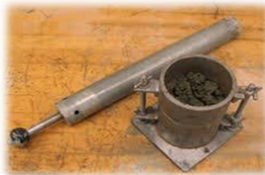
Figure 8: - Proctor compaction test apparatus
