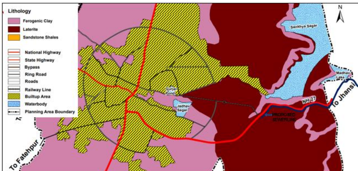
Fig. 2 shows the Lithological map showing the path of the proposed sewer line. [11]
