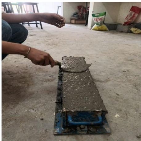
Fig.6.3: casting of beam
