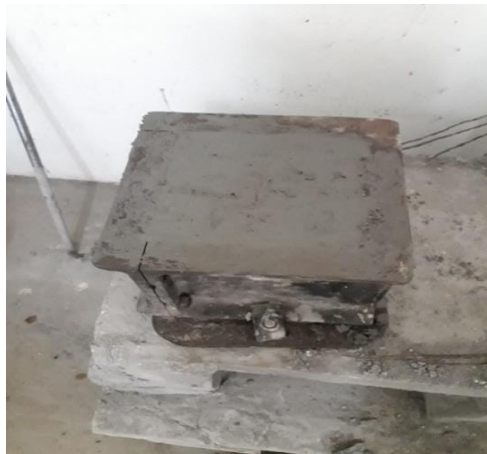
Fig.6.4: casting of cube
