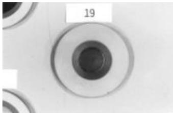
Figure 2.b. Thermal fatigue observed in post-flight coated KRS-5 sample [20]
