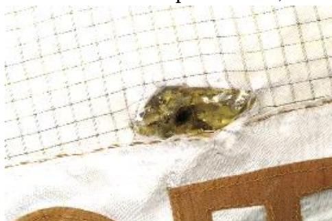
Figure 7.b. Post-flight Solar Panel Damage on Hubble, ESA [40]
