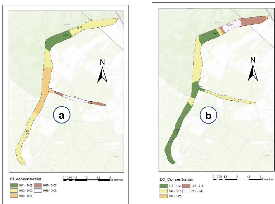
Figure 4: Spatial Distribution of \text{Cl}^- (a), EC (b), \text{HCO}_3^- (c), \text{Na}^+ (d), SAR (e) and IWQI (f) for ADW Within the Main Drainage Channel in the Study Area
