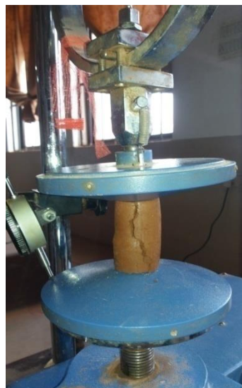
Figure 1: Shear failure after UCS test
