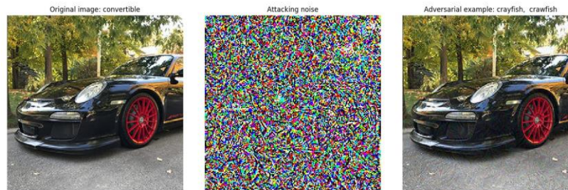
(b) Iterative non-targeted attack with \epsilon = 0.05 . The attack successfully modifies the prediction.
