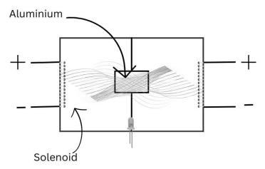
We take a container and make holes for the copper wires to be exposed and connected to the 18 volts of two 9v batteries connected in series. Keep in mind that the positive and negative terminals should match that of the diagram shown above.
