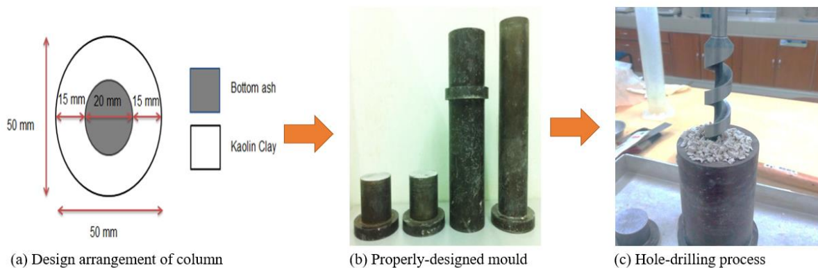
Figure 4. Bottom Ash Column Preparation Process (a) Design Arrangement of Column (b) Properly-Designed Mould (c) Hole-Drilling Process
