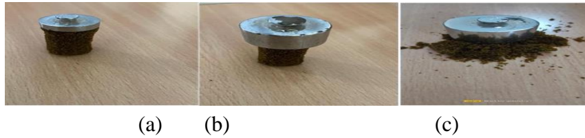
Fig:2 Strength of incense cones a) Weight of 10 gms; b) Weight of 50 gms; c) Weight of 100 gms;
