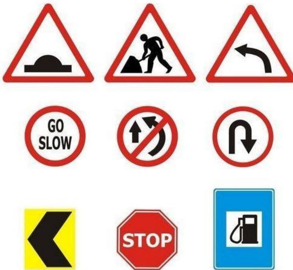
Figure 1.2 Cautionary / Warning Signs
