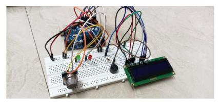
The MQ2 buzzer will take Analog value as an input value connected to A4 pin of Arduino along VCC and Ground. Piezo buzzer,16\*2 LCD,2 LED (red and green) color are Output devices connected to digital pins Arduino Uno board.
