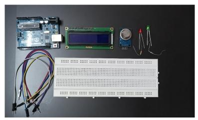
**Methodology:** This project is about a Fire and Smoke detection System when there is Smoke generated in the indoor Area of the house an Mq2 sensor will sense smoke as an Analog input value, and this is run by an Arduino program so the Output will be in digital form that is the red LED will be On, the piezo buzzer will make a sound and 1682 LCD will print the message of "ALERT!! Smoke detected".
