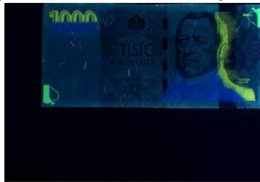
Figure 89-1000 Korun under UV light (Front)
