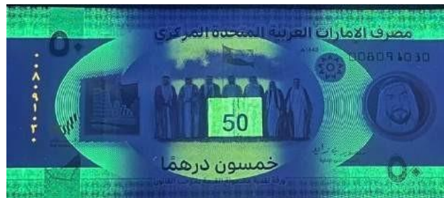
Figure 44- Latent UV Feature in 50 Dh (Back)
