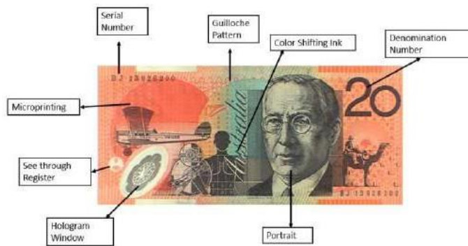
Figure 60- 20 AUD general security features (Front)
