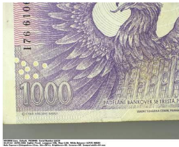
Figure 98- 1000 Korun showing OMRON rings (Back)
