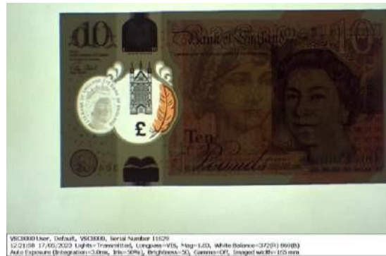
Figure 47- 10 Pounds with security features (Back)
