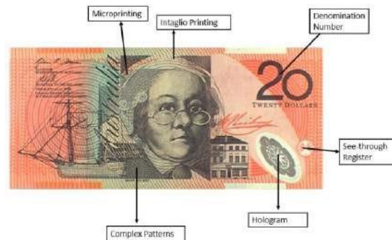
Figure 61-20 AUD general security features (Back)
