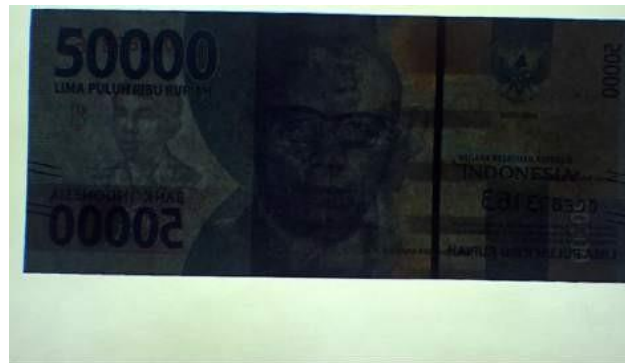
VSC3000 User, Default, VSC3000, Serial Number 11629 12/25/20 18:16:2023 Light=Transmitted, Longpass=VIS, Mag=1.89, White Balance=3720U 869RB Auto Exposure (Integration=3.2ms, Iris=50%), Brightness=50, Gamma=Off, Imaged width=150 mm
