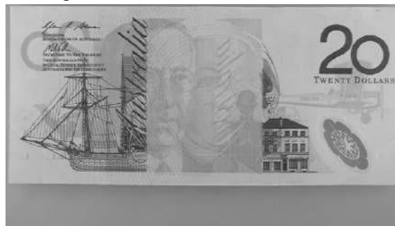
VSC3000 User, Default, VSC3000, Serial Number 11629 12/27/23 15:05:2023 Lights=IR660, Longpass=790, Mag=2.00 Auto Exposure (Integration=8ms, Iris=50%a, Brightness=50, Gamma=0ff, Image width=148 mm)
