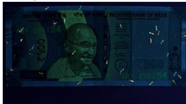
VSC3000 User, Default, VSC3000, Serial Number 11629 12-16:00 17/05/2023 Lights=365nm Ultra Violet, Longpass=0, Mag=1.00, White Balance=31 (P3.51101) Auto Exposure (Integration=500ms, Iris=50%), Brightness=50, Gamma=0.0, Imaged width=134 mm
