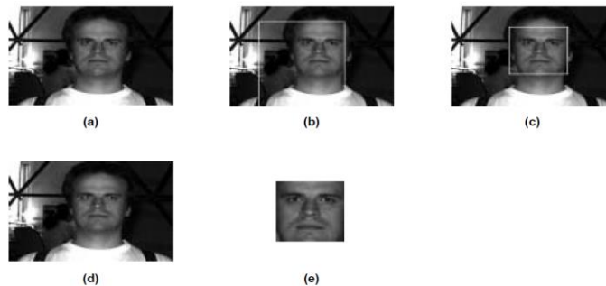
Figure 2. Face Detection, Eye Localization and Face Normalization Stages: (a) original image, (b) The box shows the reduced search space for the face after the rule-based technique is applied. At least half of the face is assumed to be inside these boundaries., (c) result of the face detection stage, (d) result of the eye localization stage, (e) normalized face image
