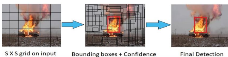
Figure 3.2.3: YOLO model approach for fire detection
