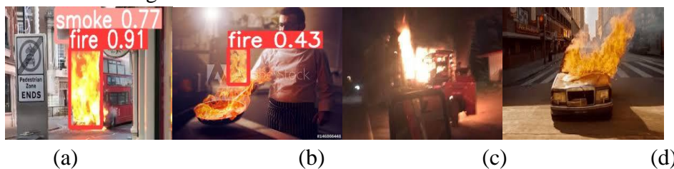
Figure 7.2: Fire Detection Results on Fire Test set Images (a) Fire Detected (TP) (b) Fire Detected (TP) (c) Fire Not Detected (FN) (d) Fire Not Detected (FN)
