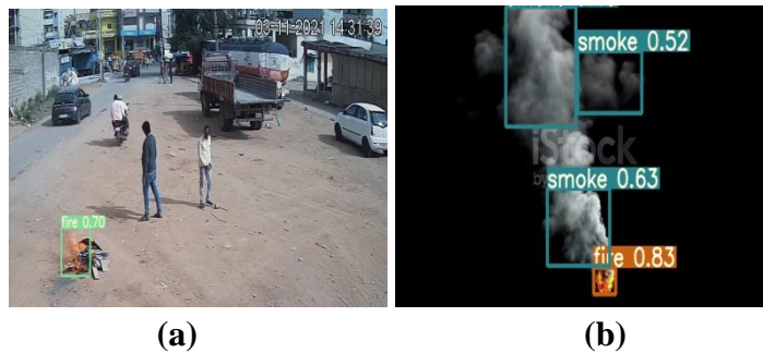
Figure 7.5: Fire & Smoke Non-Detection Results on Videos (Screenshots) (a) Fire Detected in CCTV Video Frame (b) Fire & Smoke Detected in Video Frame
