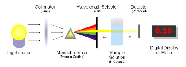
**PHOTOMETRY** Cobas c 311 analyzer is equipped with photometer to measure the absorbance of the reaction mixture in the reaction cell. The photometer lamp is located against the inner ring of the incubator bath beneth the reaction disk. The detector is outside the incubator bath ring near the cell rinse unit.
