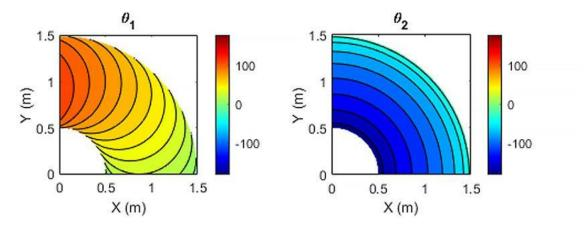
Analytic inverse kinematic solutions of the joint angles  $\theta 1$  and  $\theta 2$  at the desired end-effector pose. Robotics System Toolbox<sup>TM</sup> and Symbolic Math Toolbox<sup>TM</sup> can be used for analytical IK. With these products,
