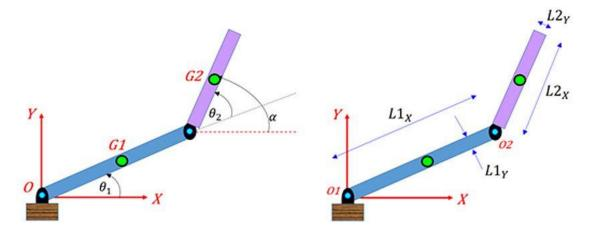
A two-linkage robot arm with the joint angles  $\theta 1$  and  $\theta 2$  and the joint parameters to calculate the inverse kinematics solutions.
