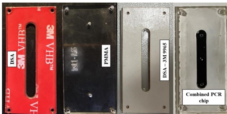
Figure 3: The fabricated PCR microchip (24 mm x 50 mm). Layers of DSA and PMMA cut with a laser cutter and combined (The channel of the combined PCR chip is filled with ink)
