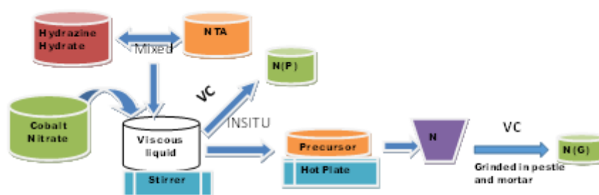
Fig. 1 Flow sheet for the preparation of Co_3O_4 (N), N(P) and N(G)
