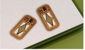
This is a living medical device that is made from human cells that secrete insulin, along with an electronic life support-system. This is a new implantable device that not only carries hundreds of thousands of insulin-producing islet cell, but also has its own on-board oxygen factory, which generate oxygen by
