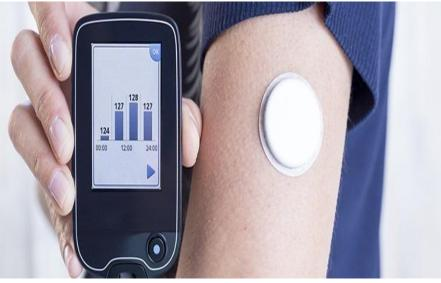
Continuous glucose monitoring means using a device to automatically estimate your blood glucose level, also called blood sugar, throughout the day and night. A continuous glucose monitor (CGM) estimates what your glucose level is every few minutes and keeps track of it over time.
