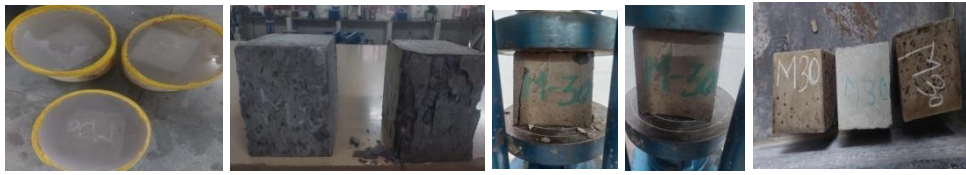
Fig- 3.5 M-30 grade concrete cubes
