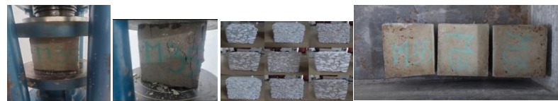
Fig- 3.14 M-35 grade concrete cubes
