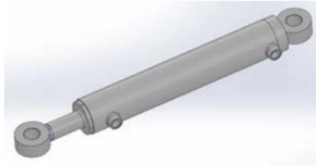
Fig. 6 Hydraulic cylinder designed for the system.
