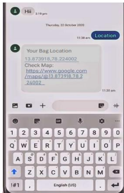
Fig (8): GSM module sent baggage location link to User through SMS
