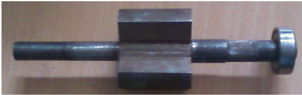
Fig 2.SRM with a tapered rotor pole (Proposed method)
