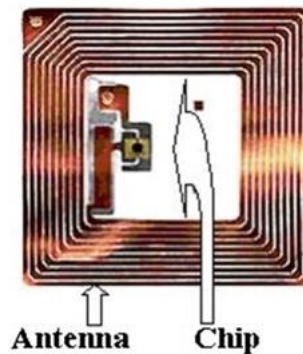
Fig. 1: RFID Tag with Chip and Antenna
