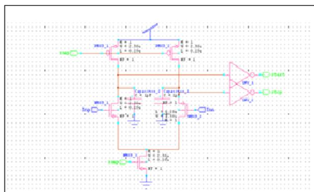
**Fig 5: Charge Steering Amplifier**
