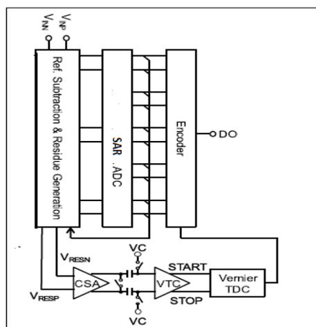
**Fig 1: Block diagram of 16-bit subranging ADC**
