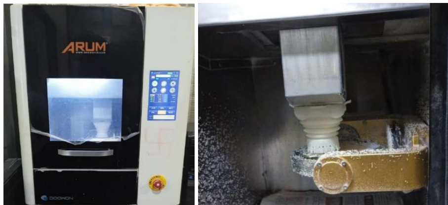
Figure no 2– Milling of CAD-CAM resin disc to form Group B samples
