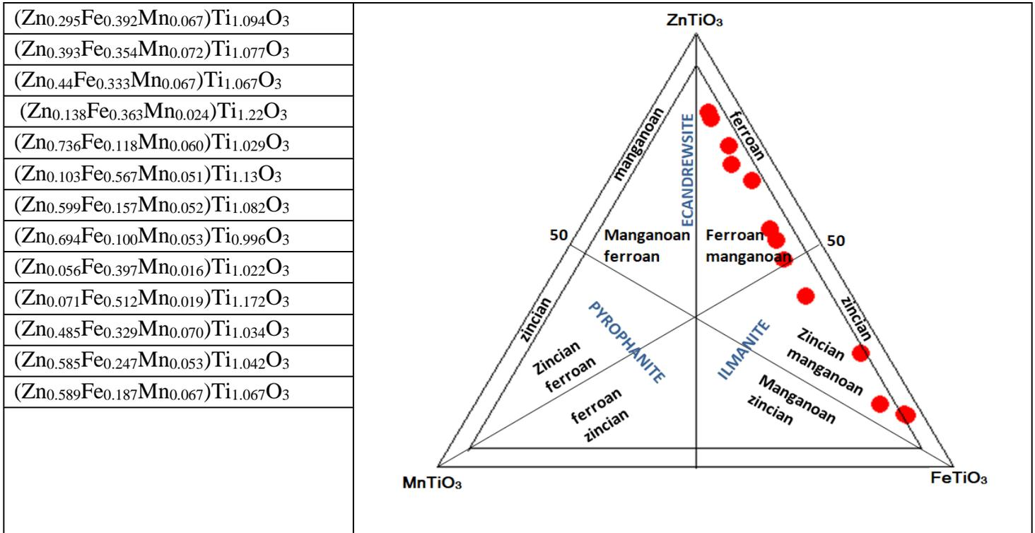
**Figure 5. Classification of Ecandrewsite and Zinc bearing Ilmenite in triangular diagram with three end members ZnTiO<sub>3</sub>-FeTiO<sub>3</sub>-MnTiO<sub>3</sub> (Mitchell & Liferovich, 2004).**
