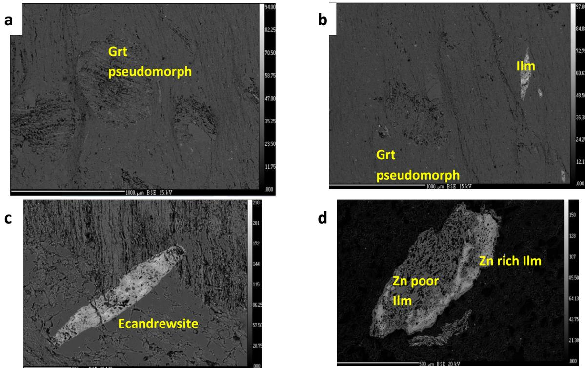
**Fig.4: BSE images showing (a) & (b) garnet pseudomorph composed of chlorite, muscovite in association with zincian ilmenite (c) & (d) euhedral grains showing exsolution between**
