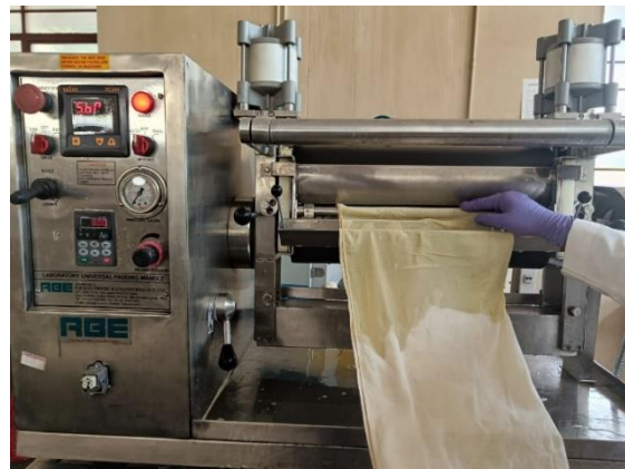
Figure 3 Coating of solution on fabric ( Padding Mangle)
