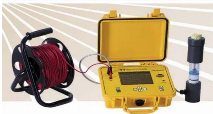
Figure 5: Half-Cell Potential test apparatus Cor Map II® (Manufacturer: James NDT)
